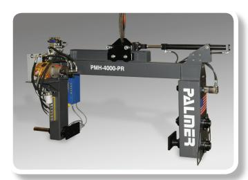
The auto-leveling feature ensures that the operator can clamp and roll a mold single-handedly. This also makes locating the clamping jaws on the mold less critical.
