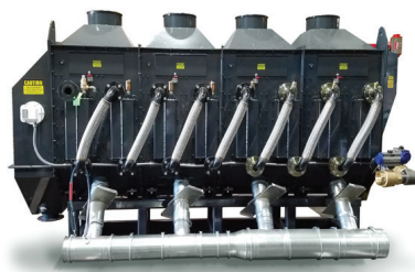
Palmer's HCCL-Series sand classifier system has four main components: a base or plenum chamber, into which fluidizing air is supplied by a blower; a fluidizing deck; a heat exchanger bundle; and a main body, which serves as a cover and pressure chamber. [PALMER MANUFACTURING & SUPPLY]
