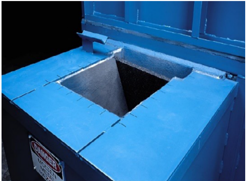
FIGURE 2: Sand foundries typically use foam filters. Ceramic or reticulated foam filters, which require greater pressure to push aluminum through, are best suited for continuous casting processes.
