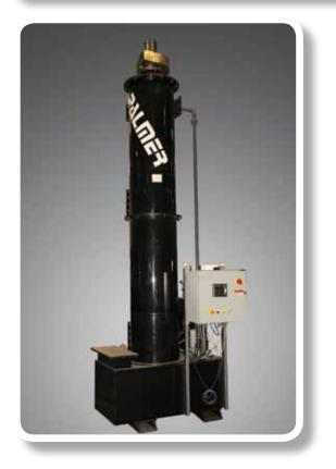
2500, 4000, 6000cfm scrubbers for Amine or S02. Scrubbers are vertical and designed for 99% removal efficiency with an inlet load-ing of 335ppm. Scrubbers require a 12' packed bed.
