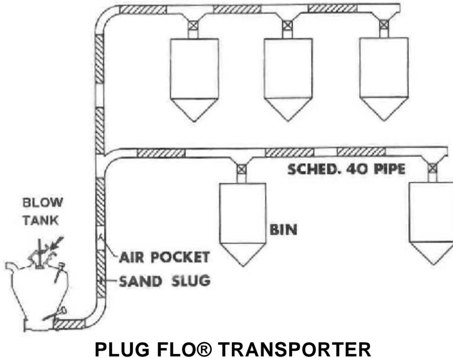
Fig. 3 Typical PLUG FLO® Sand Transporter System Layout
