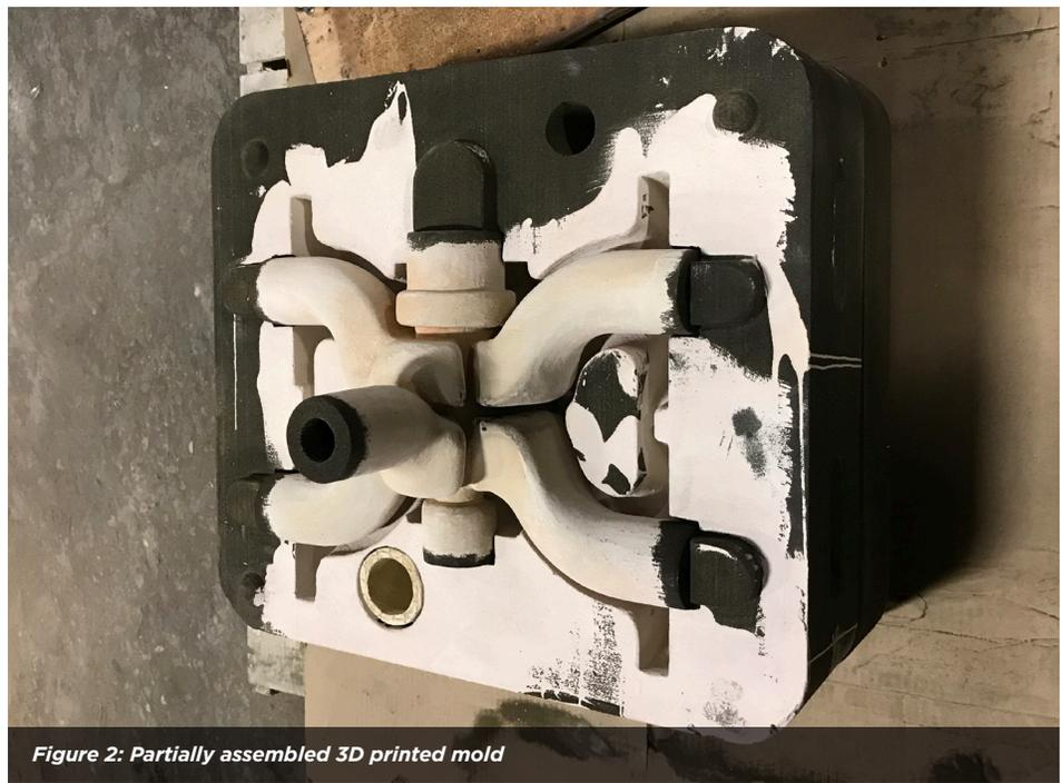
Figure 2: Partially assembled 3D printed mold
