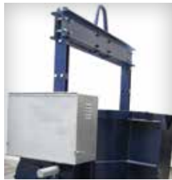
Powered Rotating Ladle
