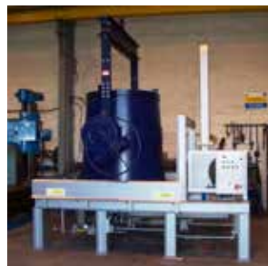
Large Bed-type Ladle Pre-Heater
