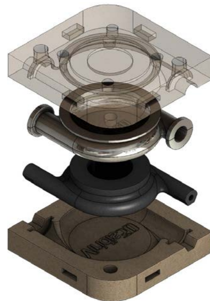
This digital rendering shows a cope, drag and core that was 3D printed on the Viridis3D RAM 123.
