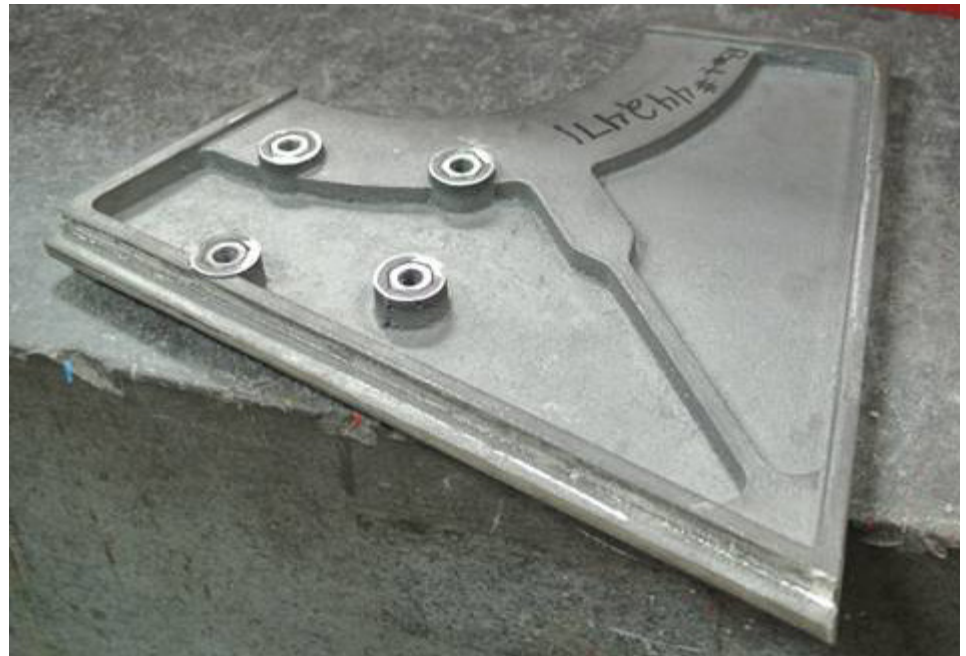
Final metalcast part using 3D printed patterns — Photo courtesy of Titan Robotics
