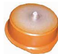
Castings Made With Reverse Tiltpour Using Riser Pour Gating
