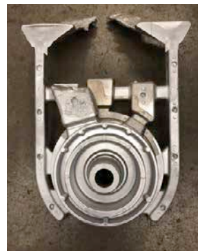
Casting Made With Traditional Tiltpour Using Parting Line Gating
