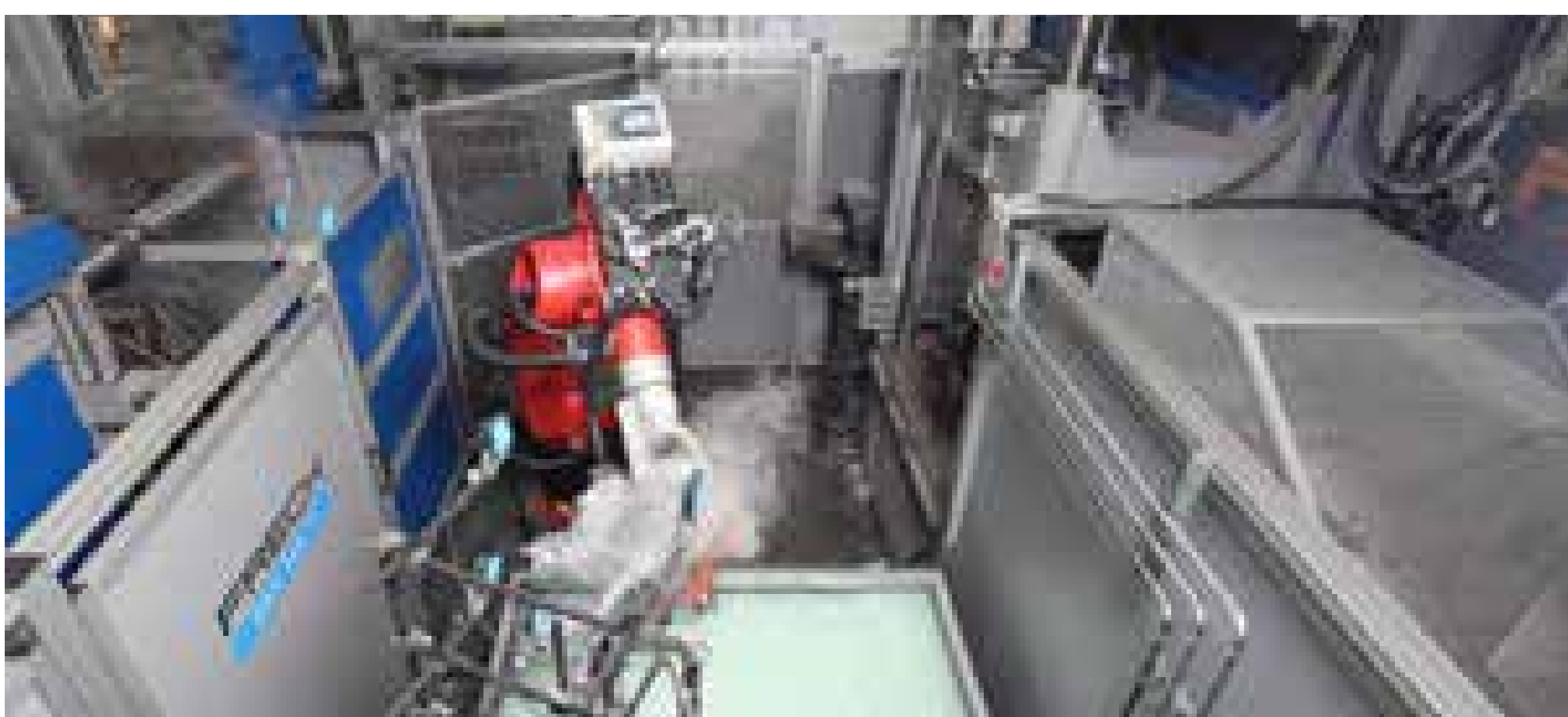
The complete product now is held by the robot into a quench tank to lower the temperature to an optimal range for further processing.
