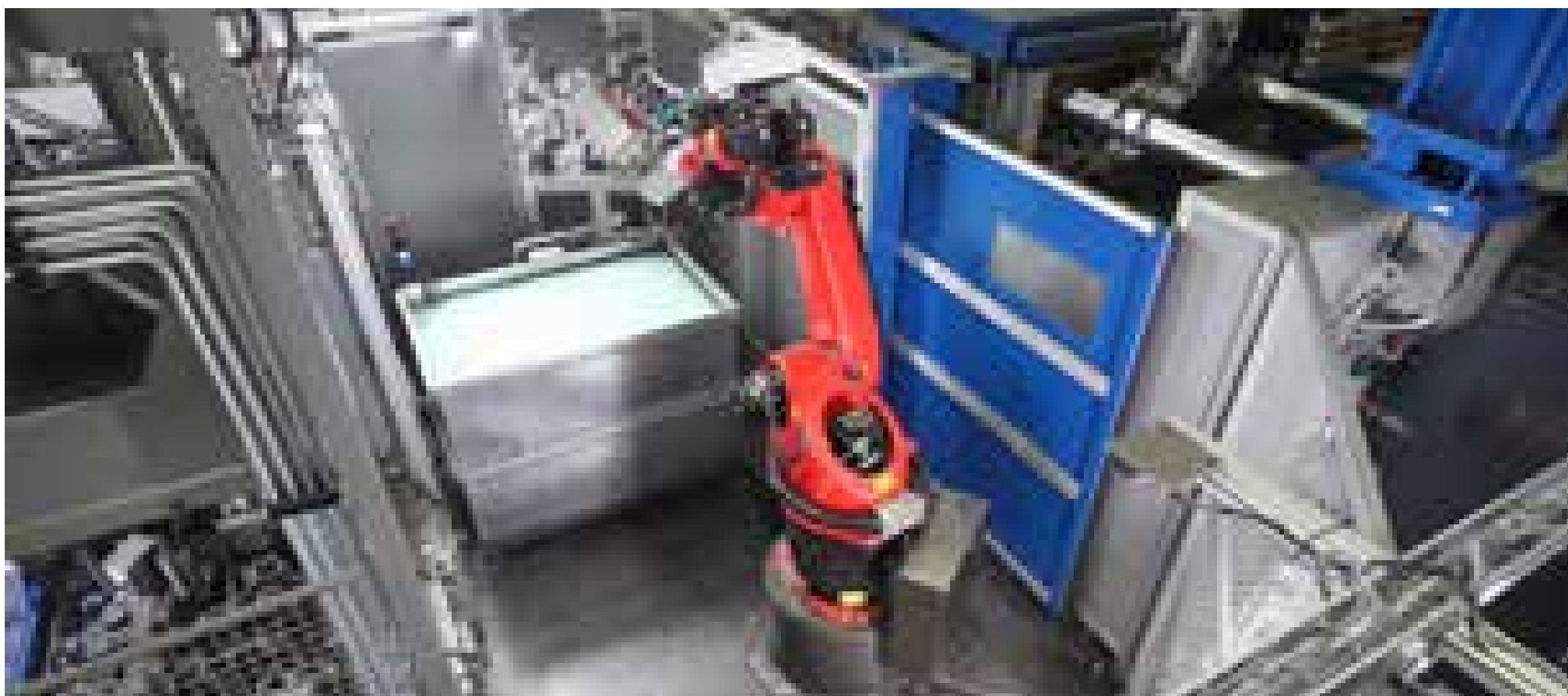
After removal from the casting machine the robot stops in front of a shot control equipped with IR sensors.
