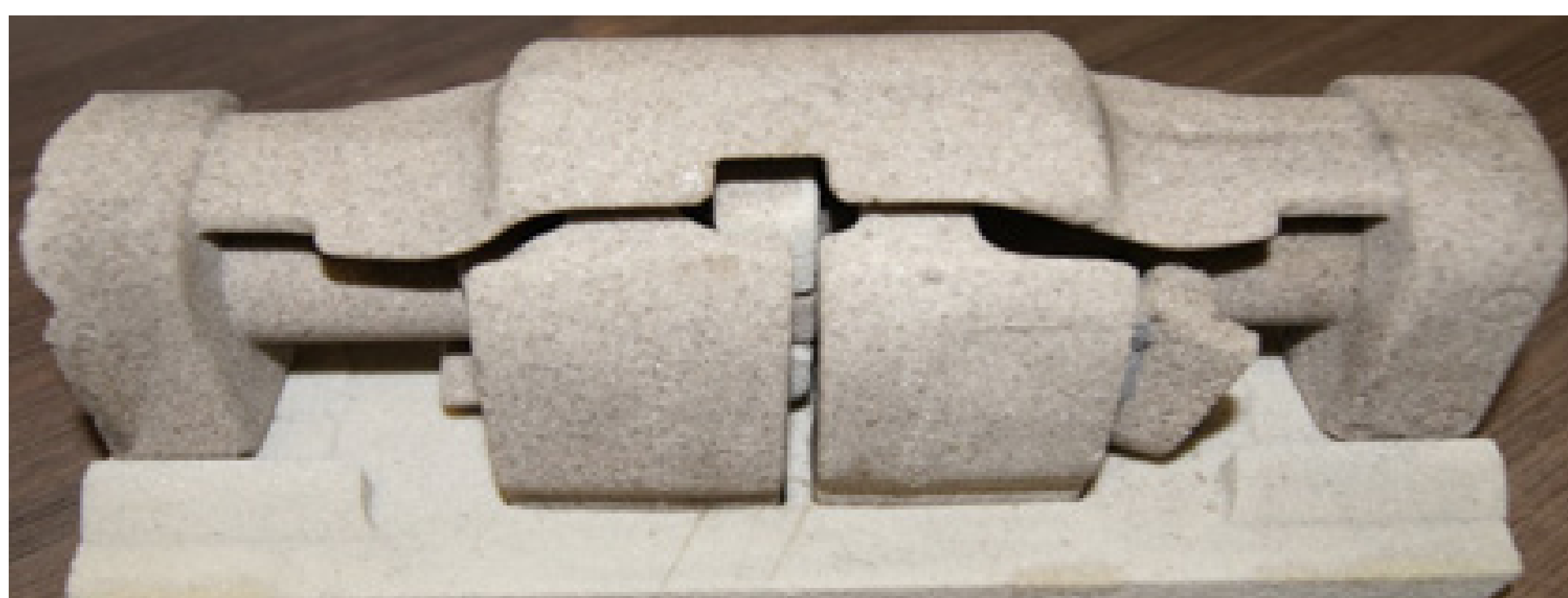
PICTURE 1. Example of a core package on a base assembled using adhesives
