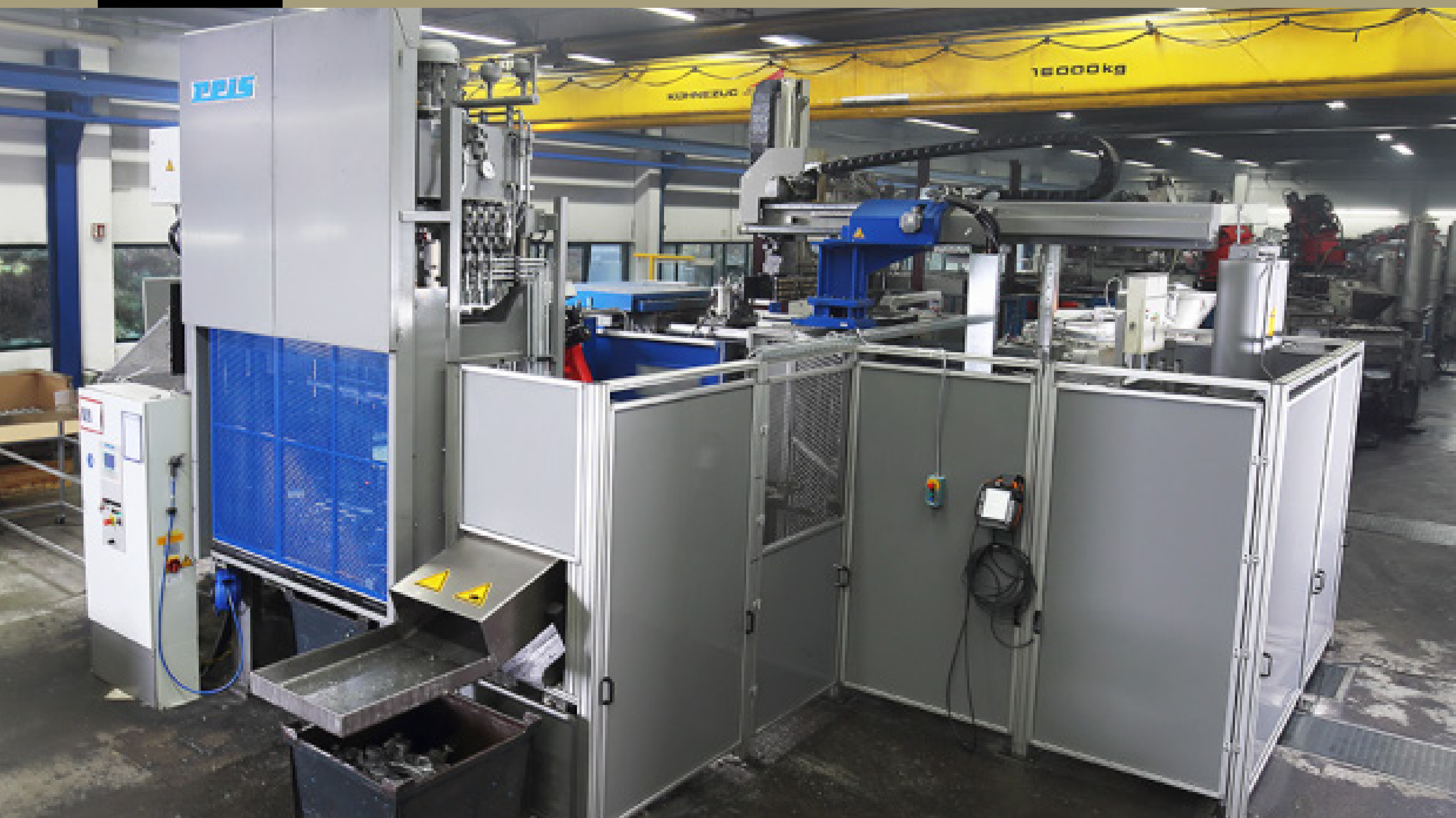
The cell comprises all steps from casting to the punch trimmed part.
