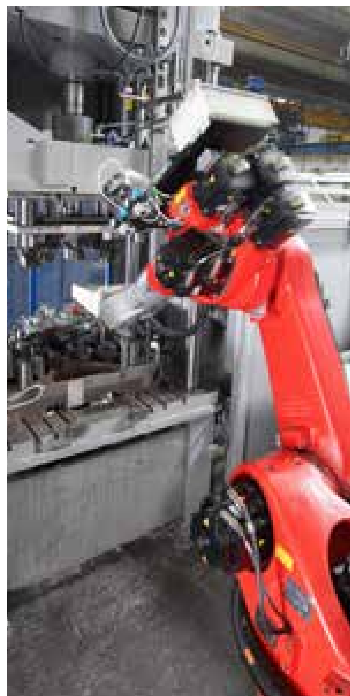
The press separates the four components and removes all casting flashes in one single work stroke.
