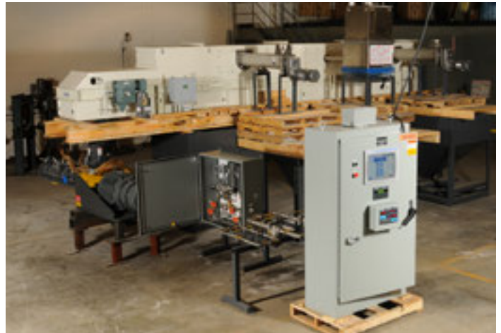
Aggregate mixing system with weigh-belt feeder
