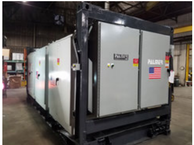
Triple mass flow pumping system (skid mounted)
